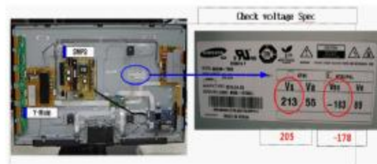
Location of Vs adjustment and test point
