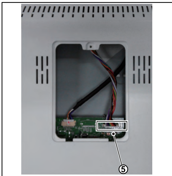
Figure 4-23 Rear cover removal[2]
