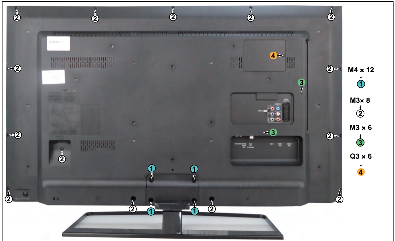
Figure 4-16 Rear cover removal[1]
