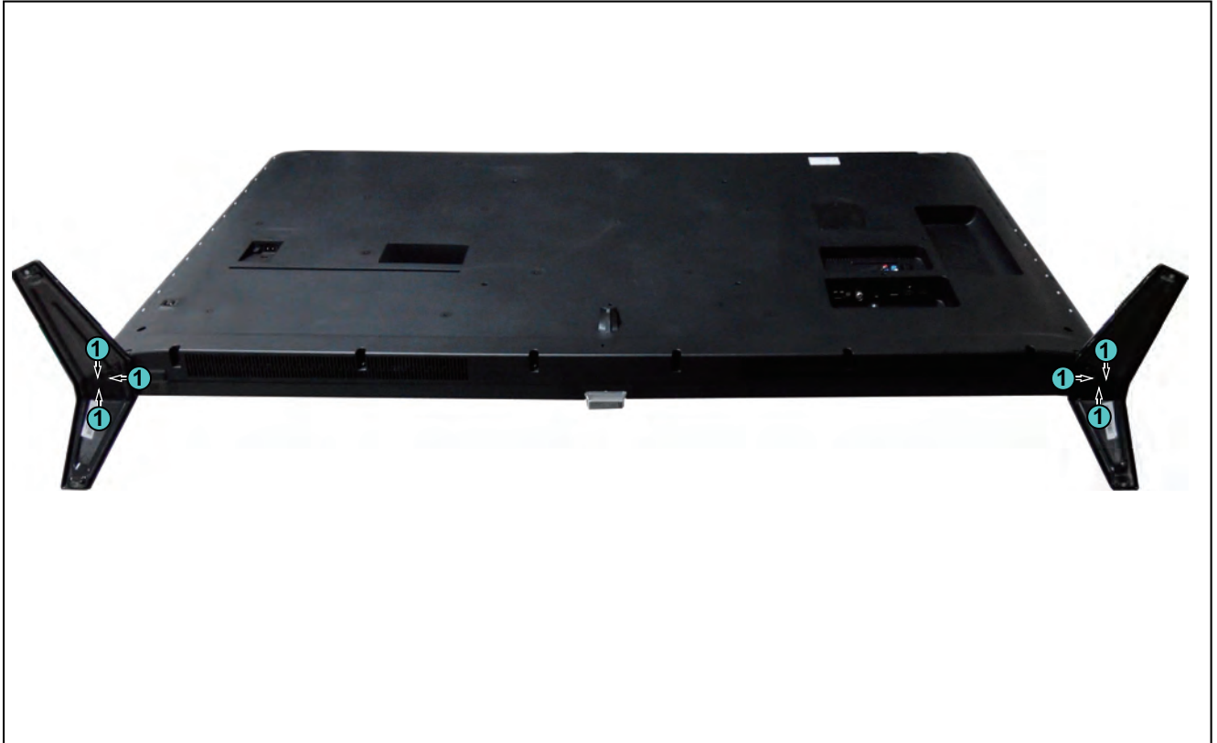
Figure 4-28 Stand removal
