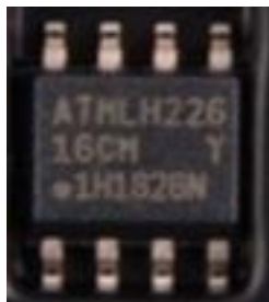
This is an Atmel 24C16 EEPROM IC
