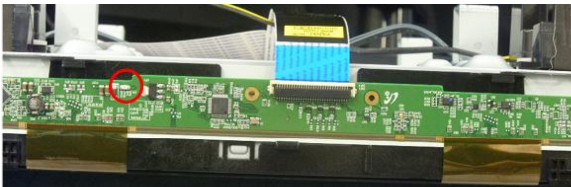
The Timing Control Section & DC-DC Circuit Built-In the LCD Panel
