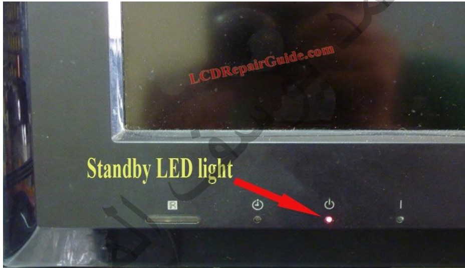
Figure B1.1: LCD TV standby LED lit and no display
