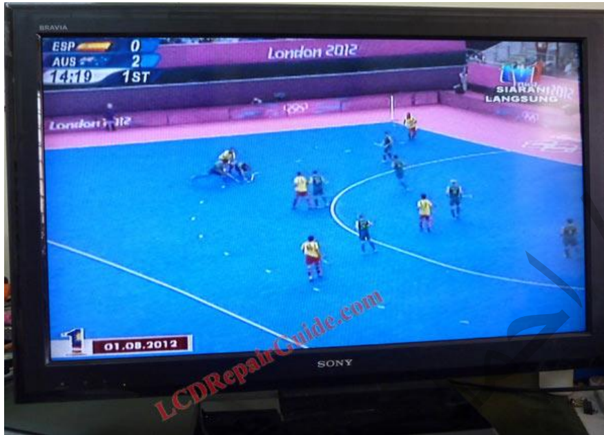
Figure B1.18: LCD TV display appeared but no sound
