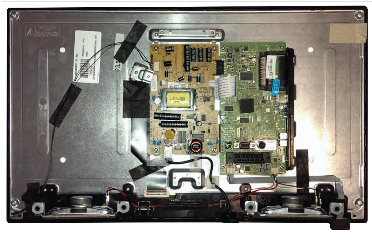
Figure 4-2 Cable dressing (24" 2000 series)
