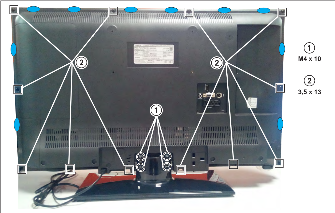
Figure 4-10 Rear cover removal (32")
