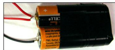
12" Wires Soldered to the +/- Battery Terminals
