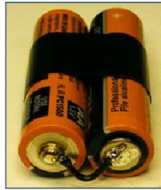
AA Batteries: +/- Soldered Together
